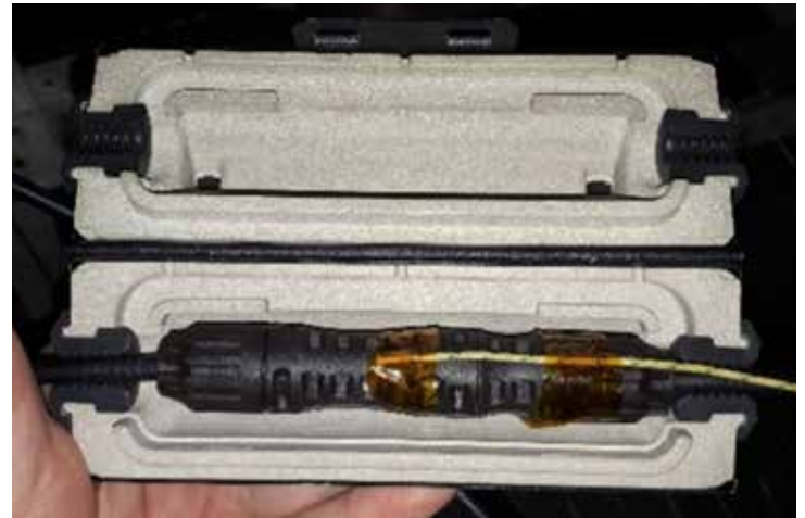
Figure 2 - ArcBox with DC Connector and thermocouple before closing
